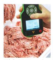
With the BFD-100 manual device from FreshDetect, bacterial contamination of minced meat can be detected in seconds.
